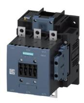
Power contactor, AC-3 150 A, 75 kW / 400 V AC (50-60 Hz) / DC operation 96-127 V UC Auxiliary contacts 2 NO + 2 NC 3-pole, Size S6 Busbar connections Drive: electronic with PLC interface 24 V DC screw terminal
