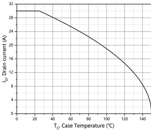
Figure 9, Drain current
