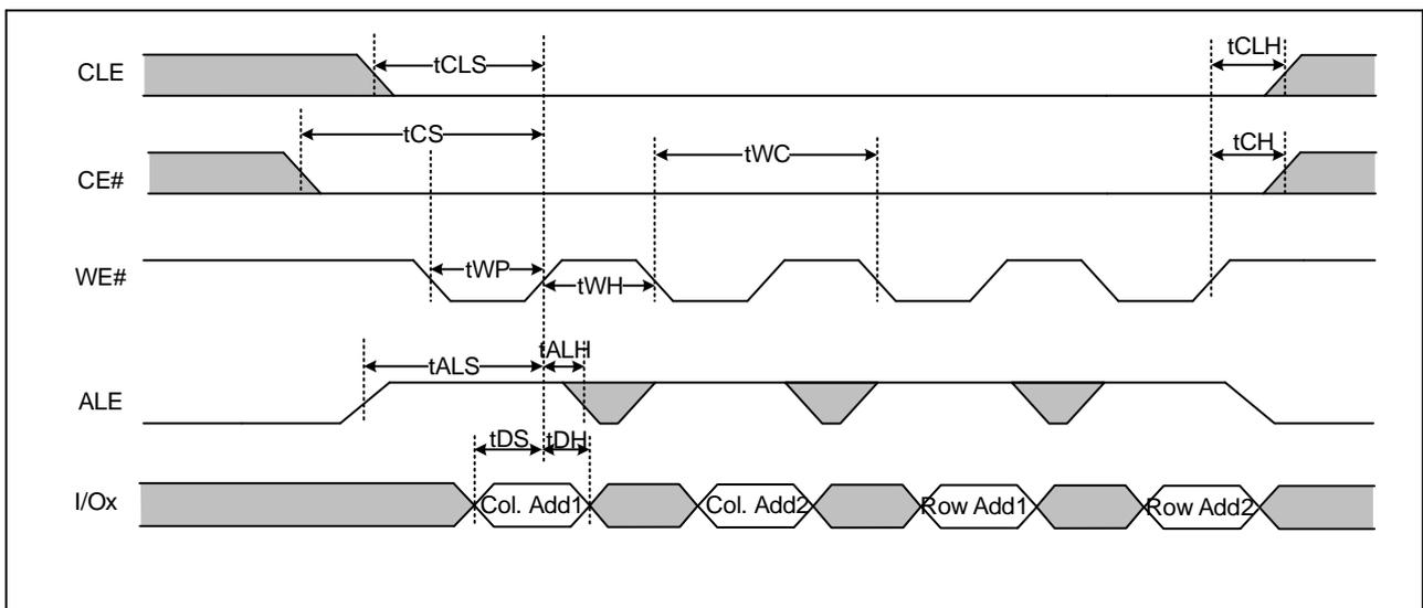
Figure 10: Address Input Cycle figures
