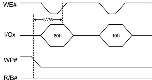
Figure 13\_b: Write Protect Enable with program figures
