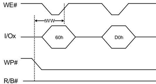
Figure 13\_d: Write Protect Enable with erase figures
