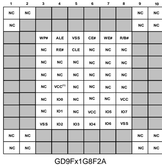
Figure 2\_b: 63-FBGA x8 device ball location figures
