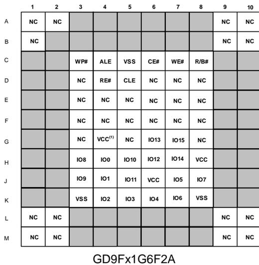
Figure 2\_a: 63-FBGA x16 device ball location figures
