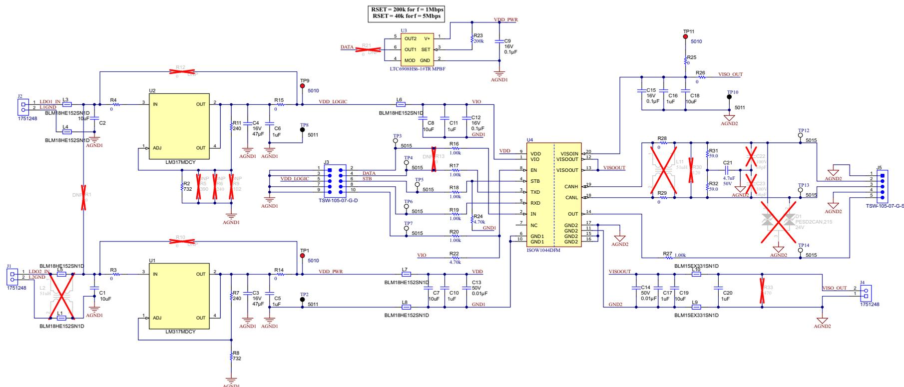
Figure 5-1. ISOW1044DFMEVM Schematic
