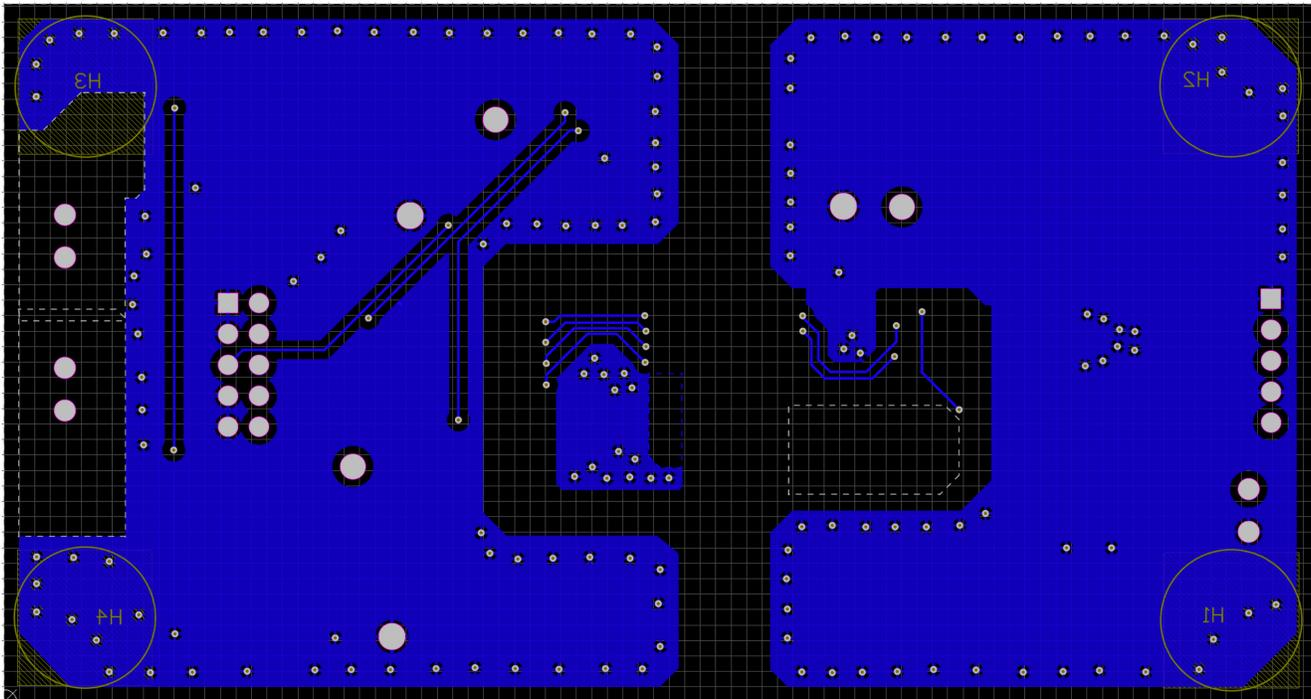
Figure 6-2. ISOW1044DFMEVM PCB Layout - Bottom Layer
