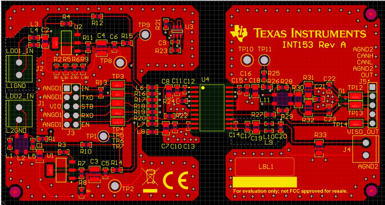
Figure 6-1. ISOW1044DFMEVM PCB Layout - Top Layer
