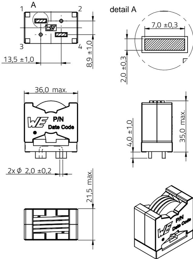
Pin 2 and 3 are only for mechanical stability and are connected to each other.
