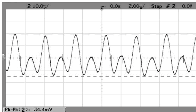
Output Ripple and Noise (Vin=5V, Vout=1.8V, Iout=3A, Cload=0, ScopeBW=100MHz)
