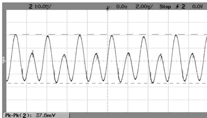
Output Ripple and Noise (Vin=5V, Vout=1.5V, Iout=3A, Cload=0, ScopeBW=100MHz)
