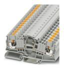
Component terminal block, If several diode terminal blocks need adding to the DIN rail, a spacer plate must be placed between them., with integrated BY255 diode, nom. voltage: 1000 V, nominal current: 1.3 A, connection method: Push-in connection, 1 level, Rated cross section: 6 mm<sup>2</sup>, cross section: 0.5 mm<sup>2</sup> - 10 mm<sup>2</sup>, color: gray
