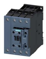
Power contactor, AC-3 40 A, 18.5 kW / 400 V 2 NO + 2 NC 83-155 V AC/DC 4-pole size S2 screw terminals 1 NO + 1 NC integrated
