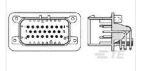
TE Part #776087-1 23POS,PIN DIA 1.3,HDR ASSY,90DEG, COD 1
