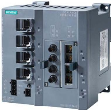
\*\*\*\*\* spare part \*\*\*\*\* SCALANCE X308-2M PoE; managed IE switch, compact; 4x 10/100/1000 Mbit/s for RJ45 ports electrical with PoE; 2x 100/1000 Mbit/s for 2-port media modules, electrical or optical; LED diagnostics, error signaling Contact with select/set pushbutton, PROFINET IO device, network management, Integrated redundancy manager, office features (RSTP, VLAN, IGMP,...) C-plug in scope of supply.
