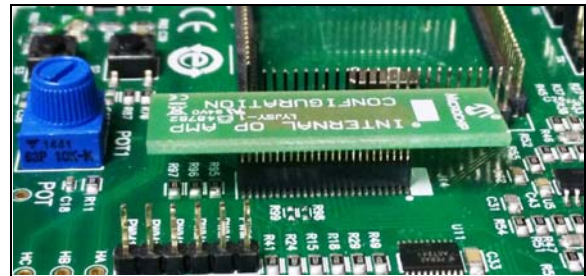
FIGURE 2: INTERNAL OP AMP CONFIGURATION BOARD
