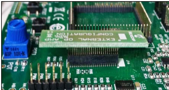
FIGURE 1: EXTERNAL OP AMP CONFIGURATION BOARD
