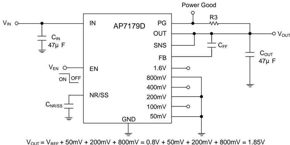
Figure 4. Output voltage set by programming pins
