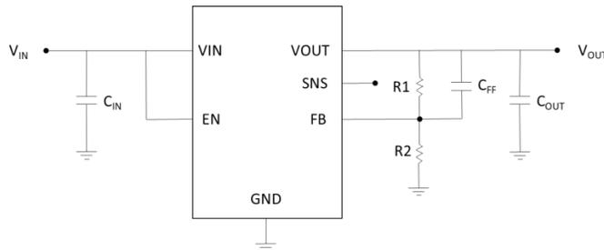
Figure 3. Output voltage set by external resistors
