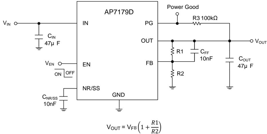
Figure 1. Configuration Circuit for V<sub>OUT</sub> Adjusted by a Resistive Divider
