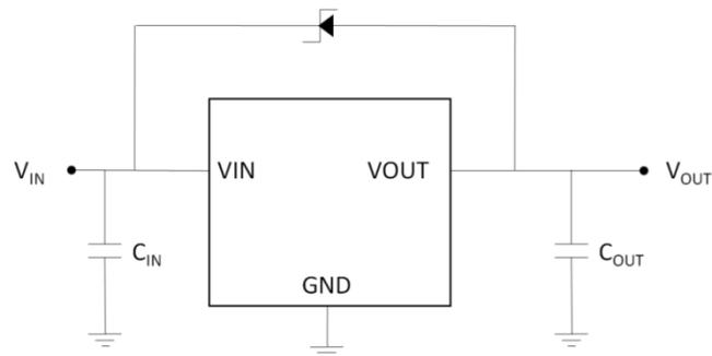
Figure 5. Application circuit for reverse current protection
