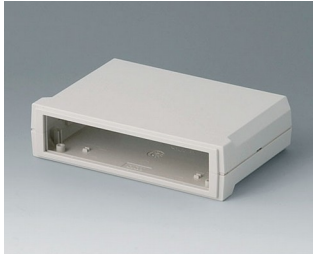
B3015117 MOTEC S, flat/flat ABS (UL 94 HB) off-white RAL 9002 6.10"x4.13"x1.57" IP 40
