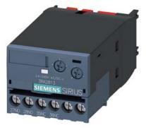
solid-state time-delayed auxiliary switch, ON-delay, relay 1 NC + 1 NO, time range 0.05-100 s, 24-240 V AC/DC, 50/60 Hz, varistor for attenuation of the contactor coils integrated, screw terminal, can be snapped onto the front on contactors 3RT20 and contactor relays 3RH2
