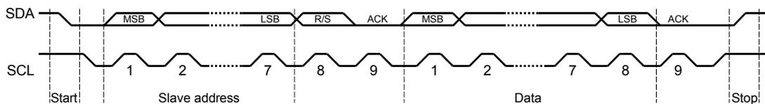
The first seven bits of the first byte make up the slave address (see Figure 16-5). The eighth bit determines the direction of the message. A zero in the R/S position of the first byte means that the master transmits (sends) data to the selected slave, and a one in this position means that the master receives data from the slave.
