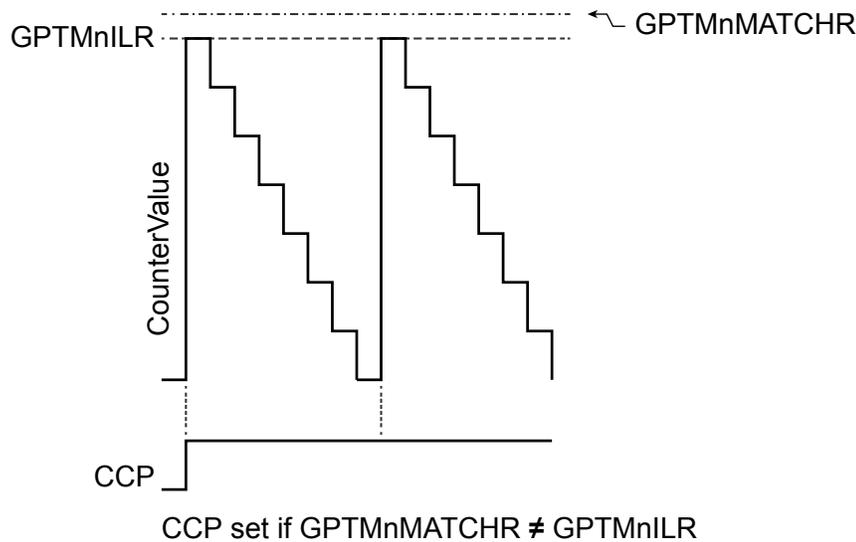
Figure 11-7 on page 710 shows how the CCP output operates when the **PLO** and **MRSU** bits are set and the **GPTMTnMATCHR** value is the same as the **GPTMTnILR** value. In this situation, if the **PLO**
