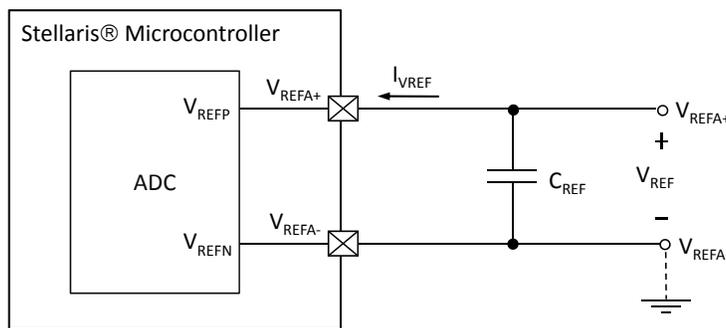
Figure 25-14. ADC Input Equivalency Diagram
