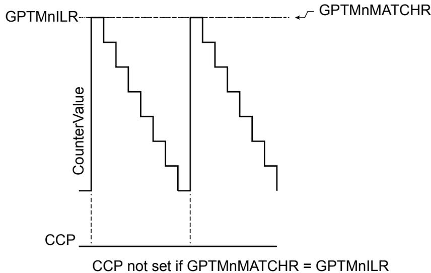
Figure 11-8 on page 710 shows how the CCP output operates when the **PLO** and **MRSU** bits are set and the **GPTMTnILR** is greater than the **GPTMTnMATCHR** value.
