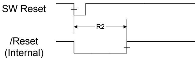
**Figure 25-10. Watchdog Reset Timing**
