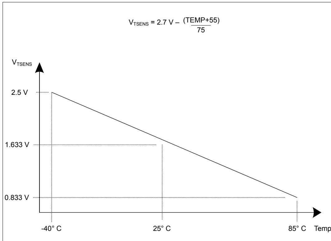
The temperature sensor reading can be sampled in a sample sequence by setting the  $TS_n$  bit in the **ADCSCTLn** register. The temperature reading from the temperature sensor can also be given as a function of the ADC value. The following formula calculates temperature (TEMP in °C) based on the ADC reading ( $ADC_{CODE}$ , given as an unsigned decimal number from 0 to 4095) and the maximum ADC voltage range ( $V_{REFP} - V_{REFN}$ ):
