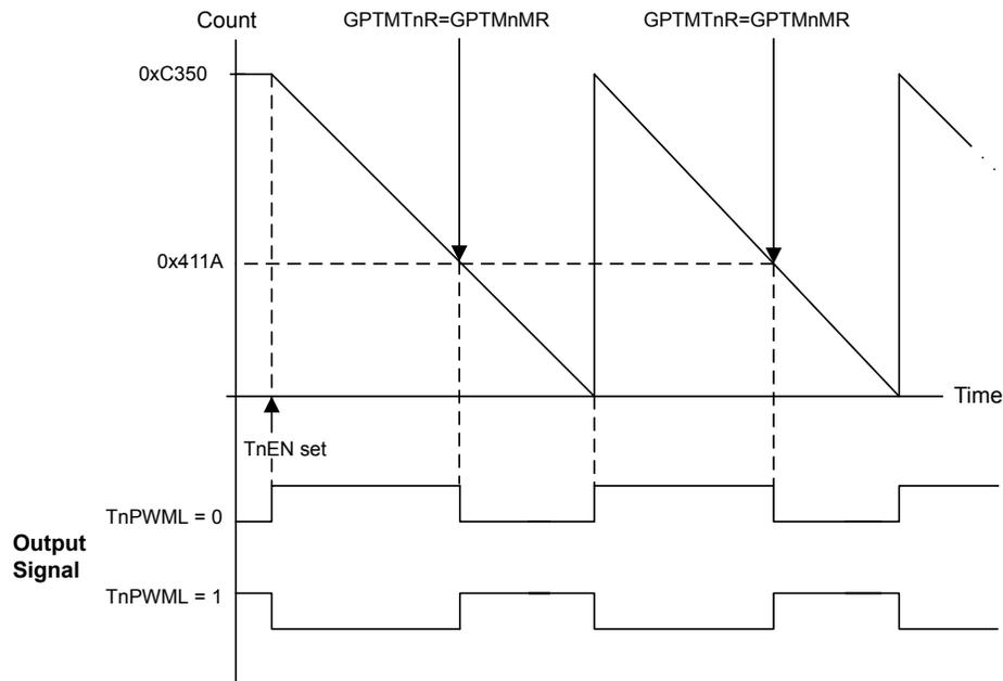
When synchronizing the timers using the **GPTMSYNC** register, the timer must be properly configured to avoid glitches on the CCP outputs. Both the **PLO** and the **MRSU** bits must be set in the **GPTMTnMR** register. Figure 11-6 on page 709 shows how the CCP output operates when the **PLO** and **MRSU** bits are set and the **GPTMTnMATCHR** value is greater than the **GPTMTnILR** value.
