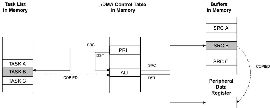
Using the channel's primary control structure, the  $\mu$ DMA controller copies task B configuration to the channel's alternate control structure.
