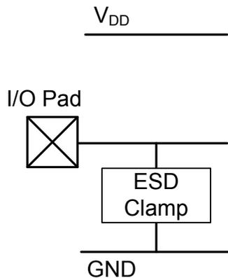
Figure 25-2 on page 1373 shows a diagram of the ESD protection on non-power, non-GPIO, and non-XOSCn pins.
