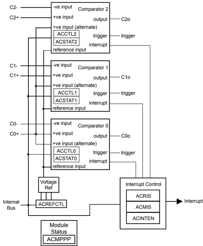
**Note:** This block diagram depicts the maximum number of analog comparators and comparator outputs for the family of microcontrollers; the number for this specific device may vary. See page 1227 for what is included on this device.
