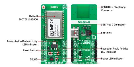
Communication between the Metis-II and the host MCU is made through a UART interface, using the standard UART RX and TX pins and hardware flow control pins (CTS/RTS). The module communicates at 115200bps by default, allowing efficient data exchange. The board includes a reset pin (RST) and a RESET button for resetting the module, and two LED indicators for user interaction: an orange TX LED signaling transmission activity and a yellow RX LED indicating reception.
