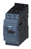
Circuit breaker size S2 for motor protection, CLASS 10 A-release 54...65 A N-release 845 A screw terminal increased switching capacity
