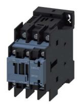
power contactor, AC-3 12 A, 5.5 kW / 400 V 1 NO + 1 NC, 24 V DC 3-pole, Size S0 ring cable lug connection
