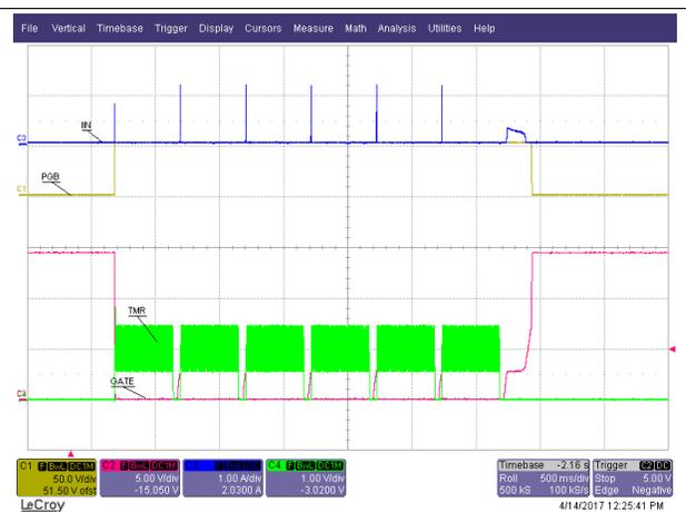
Scope Gnd = -48V\_A,  $V_{IN} = 54\text{ V}$
