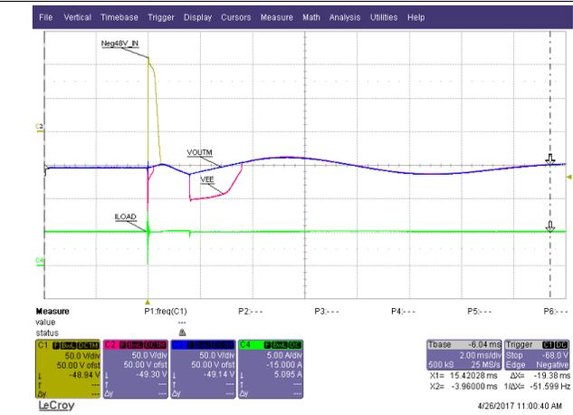
Scope GND = RTN, 5-A Load, Per IEC61000-4-5
