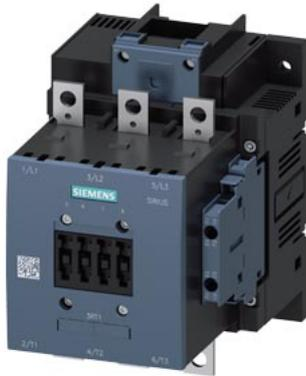
power contactor AC-1 275 A / 690 V / 40 °C 3-pole, U<sub>c</sub>: 440-480 V AC(50-60 Hz) / DC drive: conventional auxiliary contacts 2 NO + 2 NC main circuit: busbar control and auxiliary circuit: screw terminal
