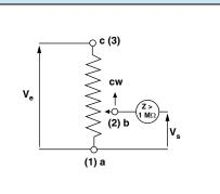
Advised load impedance: 1 M $\Omega$  min. for resistance range of 1k $\Omega$  to 50 k $\Omega$
