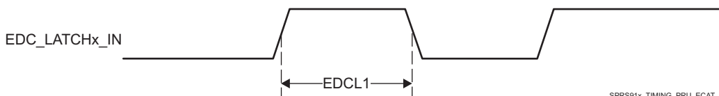
Figure 5-69. PRU-ICSS ECAT LATCHx_IN Timing
