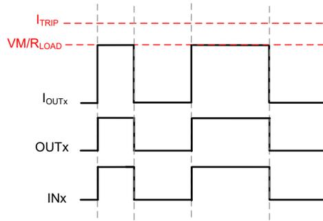
**Figure 7-3. Resistive Load Connected to ground, Cycle-by-cycle control**
