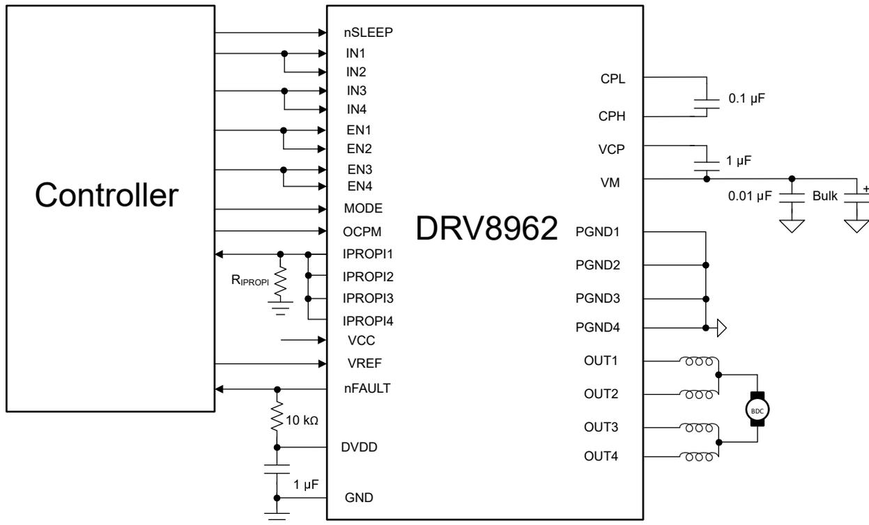
**Figure 8-7. Driving Single Brushed-DC motor with DRV8962**
