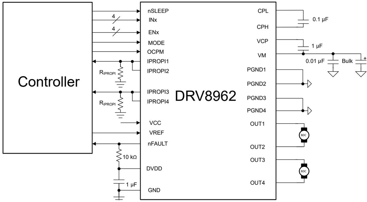
Figure 8-6. Driving two Brushed-DC Motors with DRV8962
