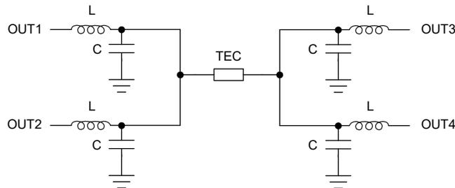
Figure 8-9. Driving one TEC with higher current
