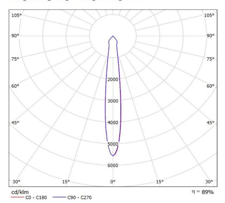
Luminaire: Ledil F14619\_ANGELETTE-S-PLAIN\_(CoB1208+TE) Lamps: 1 x Luxeon\_CoB1208\_+\_2213130-2\_+\_2213194-1\_1062.11Im@250mA\_CCT=3000K\_P=8.3007W\_I=0.25A
