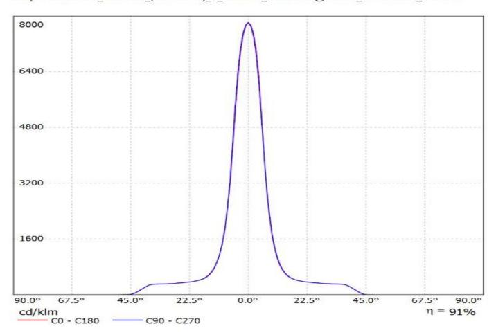
Luminaire: Ledil F14532\_ANGELETTE-S\_(CoB1208+TE) Lamps: 1 x Luxeon\_CoB1208\_+\_2213130-2\_+\_2213194-1\_1055.15lm@250mA\_CCT=3000K\_P=8.3007W\_I=0.25A
