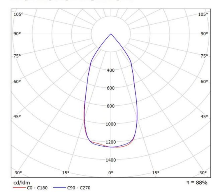
Luminaire: Ledil F14620\_ANGELETTE-M-PLAIN\_(CoB1208+TE) Lamps: 1 x Luxeon\_CoB1208\_+\_2213130-2\_+\_2213194-1\_1055.15Im@250mA\_CCT=3000K\_P=8.3007W\_I=0.25A
