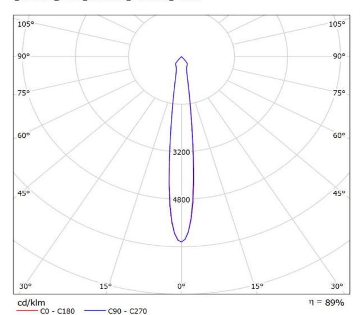
Luminaire: Ledil F14532\_ANGELETTE-S\_(CoB1208+IDEAL) Lamps: 1 x Luxeon\_CoB1208\_+\_50-2100SH+50-2100AN\_1062.11Im@250mA\_CCT=3000K\_P=8.3007W\_I=0.25A
