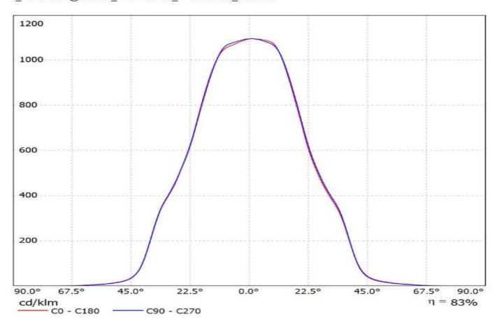
Luminaire: Ledil FN15268\_ANGELETTE-M-RZ\_(CoB1208+TE) Lamps: 1 x Luxeon\_CoB1208\_+\_2213130-2\_+\_2213194-1\_1055.15lm@250mA\_CCT=3000K\_P=8.3007W\_I=0.25A
