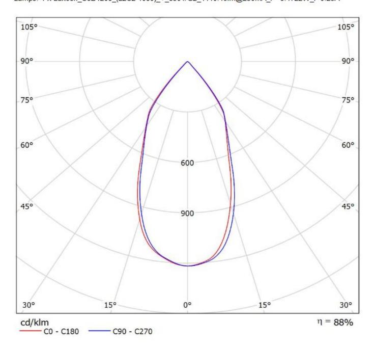
Luminaire: Ledil FN15268\_ANGELETTE-M-RZ\_(CoB1208+TE) Lamps: 1 x Luxeon\_CoB1208\_+\_2213130-2\_+\_2213194-1\_1055.15Im@250mA\_CCT=3000K\_P=8.3007W\_I=0.25A
