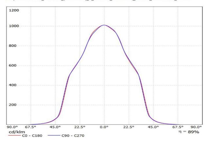
Luminaire: Ledil FN15269\_ANGELETTE-WW-RZ\_(CoB1208+TE) Lamps: 1 x Luxeon\_CoB1208\_+\_2213130-2\_+\_2213194-1\_1055.15Im@250mA\_CCT=3000K\_P=8.3007W\_I=0.25A
