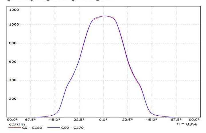
Luminaire: Ledil F14534\_ANGELETTE-WW\_(CoB1208+IDEAL) Lamps: 1 x Luxeon\_CoB1208\_+\_50-2100SH+50-2100AN\_1062.11Im@250mA\_CCT=3000K\_P=8.3007W\_I=0.25A
