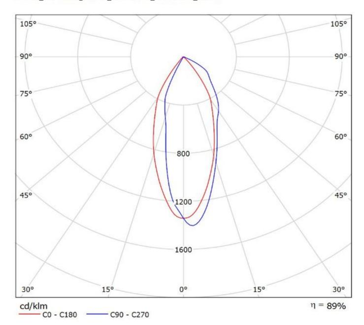
Luminaire: Ledil C14346\_ANGELETTE-WAS\_(CoB1208+TE) Lamps: 1 x Luxeon\_CoB1208\_+\_2213130-2\_+\_2213194-1\_1062.11Im@250mA\_CCT=3000K\_P=8.3007W\_I=0.25A
