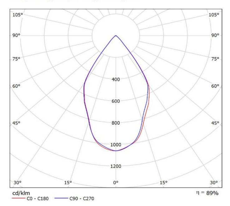
Luminaire: Ledil F14534\_ANGELETTE-WW\_(CoB1208+TE) Lamps: 1 x Luxeon\_CoB1208\_+\_2213130-2\_+\_2213194-1\_1062.11Im@250mA\_CCT=3000K\_P=8.3007W\_l=0.25A
