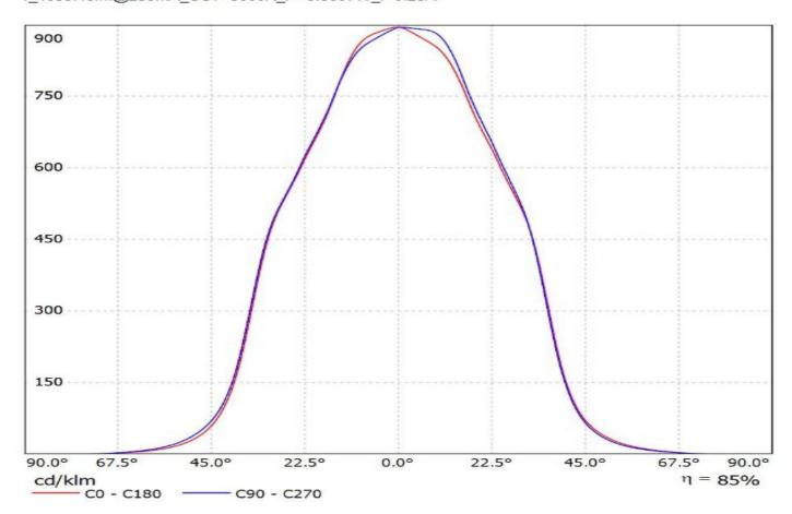
Luminaire: Ledil FN15272\_ANGELETTE-WW-PLAIN-RZ\_(CoB1208+TE) Lamps: 1 x Luxeon\_CoB1208\_+\_2213130-2\_+\_2213194-1\_1055.15Im@250mA\_CCT=3000K\_P=8.3007W\_I=0.25A
