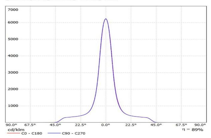
Luminaire: Ledil F14532\_ANGELETTE-S\_(CoB1208+IDEAL) Lamps: 1 x Luxeon\_CoB1208\_+\_50-2100SH+50-2100AN\_1062.11Im@250mA\_CCT=3000K\_P=8.3007W\_I=0.25A
