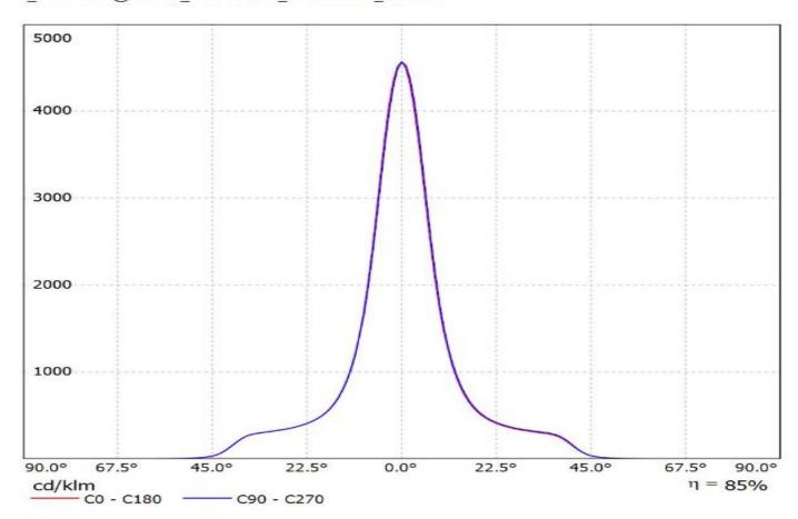
Luminaire: Ledil FN15270\_ANGELETTE-S-PLAIN-RZ\_(CoB1208+TE) Lamps: 1 x Luxeon\_CoB1208\_+\_2213130-2\_+\_2213194-1\_1055.15Im@250mA\_CCT=3000K\_P=8.3007W\_I=0.25A
