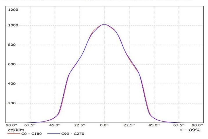
Luminaire: Ledil FN15272\_ANGELETTE-WW-PLAIN-RZ\_(CoB1208+IDEAL) Lamps: 1 x Luxeon\_CoB1208\_+\_50-2100SH+50-2100AN\_1062.11Im@250mA\_CCT=3000K\_P=8.3007W\_I=0.25A
