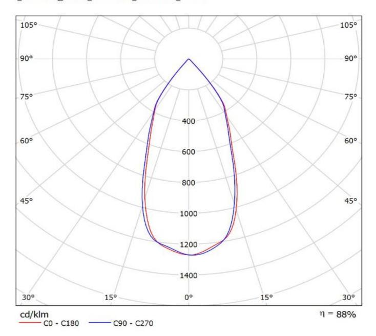
Luminaire: Ledil F14533\_ANGELETTE-M\_(CoB1208+TE) Lamps: 1 x Luxeon\_CoB1208\_+\_2213130-2\_+\_2213194-1\_1062.11Im@250mA\_CCT=3000K\_P=8.3007W\_I=0.25A
