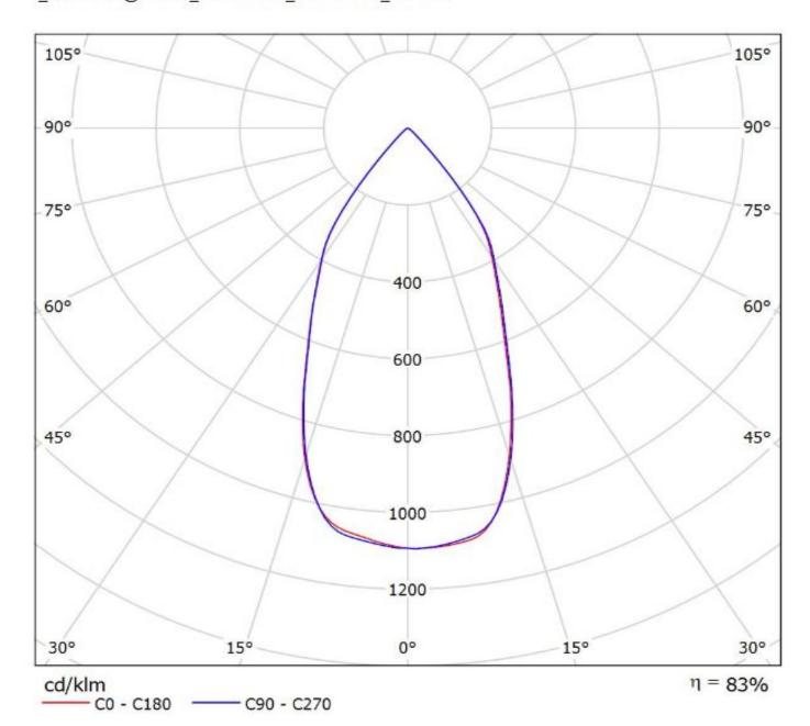
Luminaire: Ledil FN15268\_ANGELETTE-M-RZ\_(CoB1208+TE) Lamps: 1 x Luxeon\_CoB1208\_+\_2213130-2\_+\_2213194-1\_1055.15Im@250mA\_CCT=3000K\_P=8.3007W\_I=0.25A
