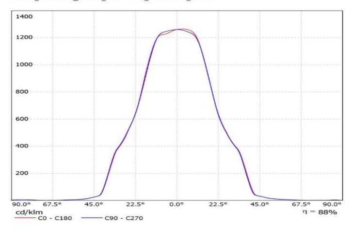
Luminaire: Ledil F14620\_ANGELETTE-M-PLAIN\_(CoB1208+TE) Lamps: 1 x Luxeon\_CoB1208\_+\_2213130-2\_+\_2213194-1\_1055.15Im@250mA\_CCT=3000K\_P=8.3007W\_I=0.25A
