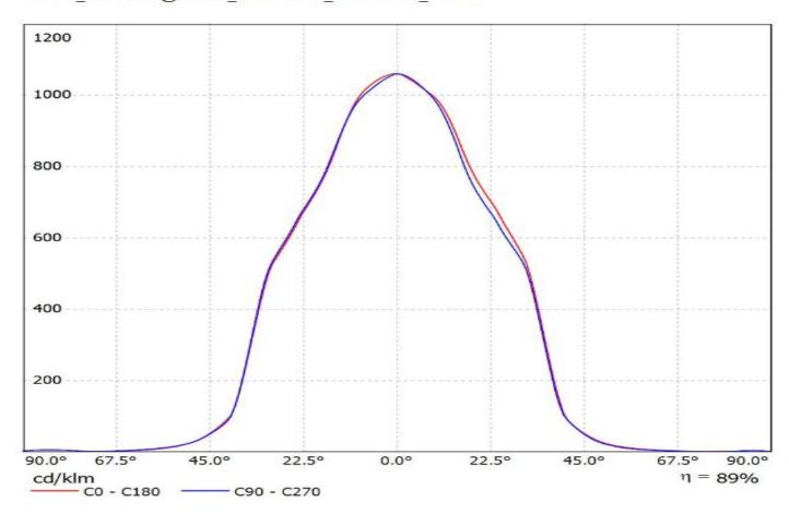
Luminaire: Ledil F14622\_ANGELETTE-WW-PLAIN\_(CoB1208+TE) Lamps: 1 x Luxeon\_CoB1208\_+\_2213130-2\_+\_2213194-1\_1055.15Im@250mA\_CCT=3000K\_P=8.3007W\_I=0.25A
