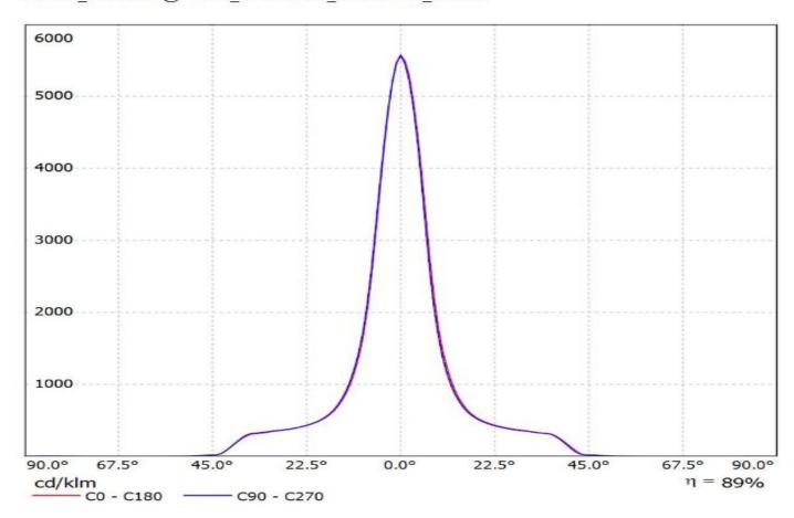
Luminaire: Ledil F14619\_ANGELETTE-S-PLAIN\_(CoB1208+IDEAL) Lamps: 1 x Luxeon\_CoB1208\_+\_50-2100SH+50-2100AN\_1062.11Im@250mA\_CCT=3000K\_P=8.3007W\_I=0.25A
