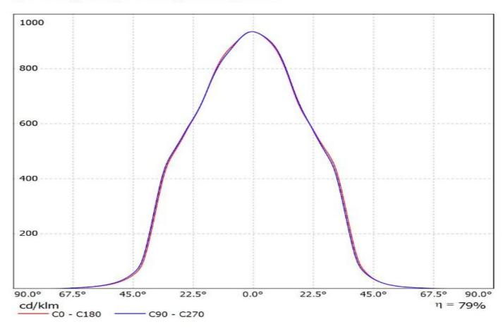
Luminaire: Ledil F14622\_ANGELETTE-WW-PLAIN\_(CoB1208+IDEAL) Lamps: 1 x Luxeon\_CoB1208\_+\_50-2100SH+50-2100AN\_1062.11Im@250mA\_CCT=3000K\_P=8.3007W\_I=0.25A
