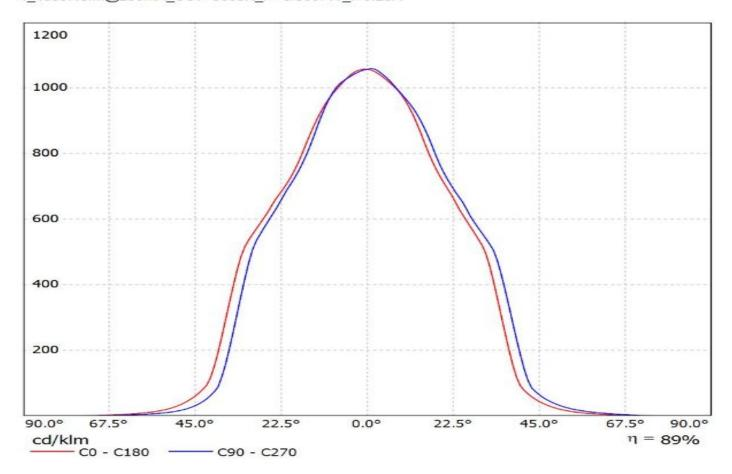
Luminaire: Ledil F14534\_ANGELETTE-WW\_(CoB1211+IDEAL) Lamps: 1 x Luxeon\_CoB1211\_(L2C2-4080)\_50-2204CT+50-2100AN\_1376.18Im@250mA\_P=7.9988W\_I=0.25A
