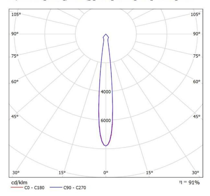
Luminaire: Ledil F14532\_ANGELETTE-S\_(CoB1208+TE) Lamps: 1 x Luxeon\_CoB1208\_+\_2213130-2\_+\_2213194-1\_1055.15lm@250mA\_CCT=3000K\_P=8.3007W\_I=0.25A
