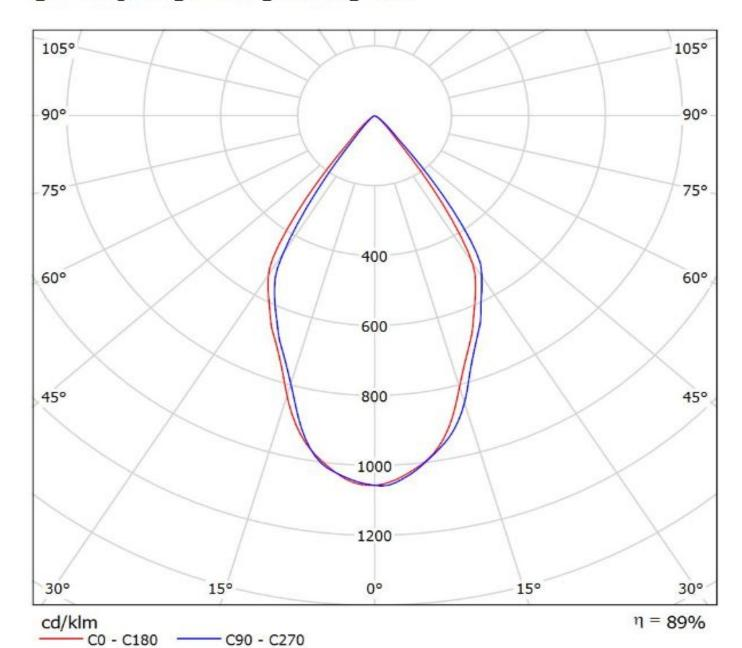
Luminaire: Ledil F14534\_ANGELETTE-WW\_(CoB1211+IDEAL) Lamps: 1 x Luxeon\_CoB1211\_(L2C2-4080)\_50-2204CT+50-2100AN\_1376.18Im@250mA\_P=7.9988W\_I=0.25A
