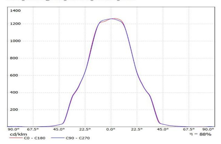
Luminaire: Ledil F14620\_ANGELETTE-M-PLAIN\_(CoB1208+IDEAL) Lamps: 1 x Luxeon\_CoB1208\_+\_50-2100SH+50-2100AN\_1062.11Im@250mA\_CCT=3000K\_P=8.3007W\_I=0.25A
