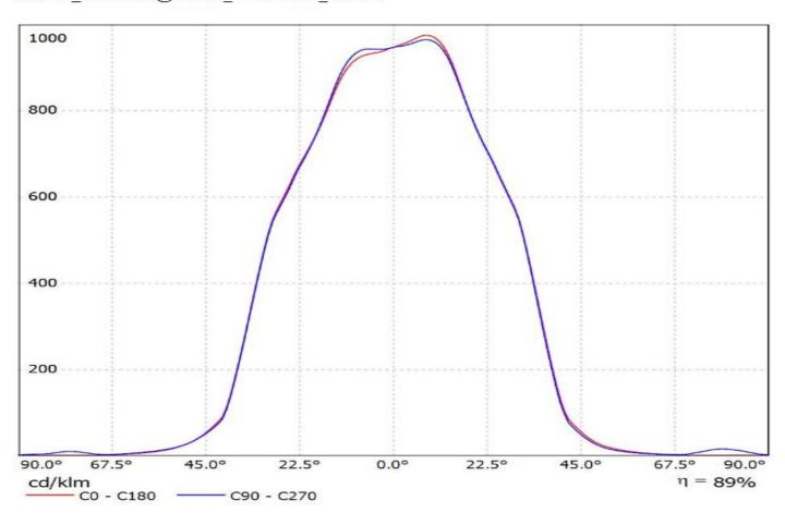
Luminaire: Ledil FN15269\_ANGELETTE-WW-RZ\_(CoB1208+IDEAL) Lamps: 1 x Luxeon\_CoB1208\_+\_50-2100SH+50-2100AN\_1062.11Im@250mA\_CCT=3000K\_P=8.3007W\_I=0.25A
