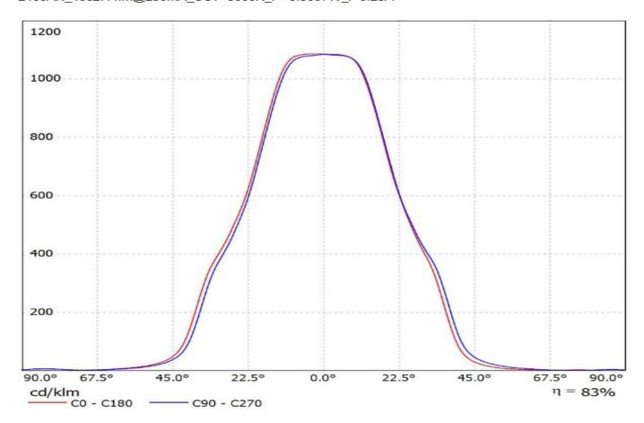
Luminaire: Ledil FN15271\_ANGELETTE-M-PLAIN-RZ\_(CoB1208+TE) Lamps: 1 x Luxeon\_CoB1208\_+\_2213130-2\_+\_2213194-1\_1055.15Im@250mA\_CCT=3000K\_P=8.3007W\_I=0.25A
