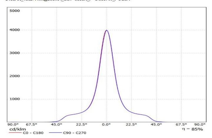
Luminaire: Ledil F14533\_ANGELETTE-M\_(CoB1208+IDEAL) Lamps: 1 x Luxeon\_CoB1208\_+\_50-2100SH+50-2100AN\_1062.11Im@250mA\_CCT=3000K\_P=8.3007W\_I=0.25A
