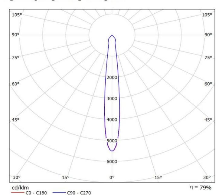
Luminaire: Ledil FN15267\_ANGELETTE-S-RZ\_(CoB1208+TE) Lamps: 1 x Luxeon\_CoB1208\_+\_2213130-2\_+\_2213194-1\_1055.15Im@250mA\_CCT=3000K\_P=8.3007W\_I=0.25A
