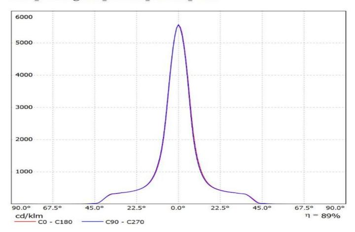
Luminaire: Ledil F14619\_ANGELETTE-S-PLAIN\_(CoB1208+TE) Lamps: 1 x Luxeon\_CoB1208\_+\_2213130-2\_+\_2213194-1\_1062.11Im@250mA\_CCT=3000K\_P=8.3007W\_I=0.25A
