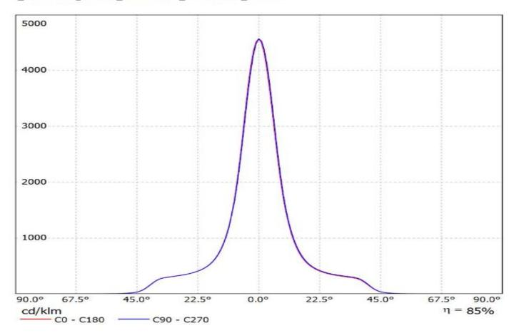
Luminaire: Ledil FN15267\_ANGELETTE-S-RZ\_(CoB1208+IDEAL) Lamps: 1 x Luxeon\_CoB1208\_+\_50-2100SH+50-2100AN\_1062.11Im@250mA\_CCT=3000K\_P=8.3007W\_I=0.25A
