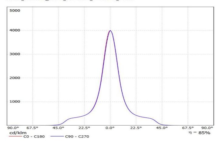
Luminaire: Ledil FN15270\_ANGELETTE-S-PLAIN-RZ\_(CoB1208+IDEAL) Lamps: 1 x Luxeon\_CoB1208\_+\_50-2100SH+50-2100AN\_1062.11Im@250mA\_CCT=3000K\_P=8.3007W\_I=0.25A
