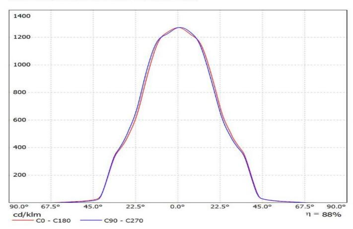
Luminaire: Ledil F14533\_ANGELETTE-M\_(CoB1208+TE) Lamps: 1 x Luxeon\_CoB1208\_+\_2213130-2\_+\_2213194-1\_1062.11Im@250mA\_CCT=3000K\_P=8.3007W\_I=0.25A
