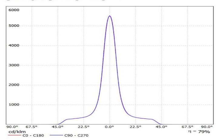
Luminaire: Ledil FN15267\_ANGELETTE-S-RZ\_(CoB1208+TE) Lamps: 1 x Luxeon\_CoB1208\_+\_2213130-2\_+\_2213194-1\_1055.15Im@250mA\_CCT=3000K\_P=8.3007W\_I=0.25A
