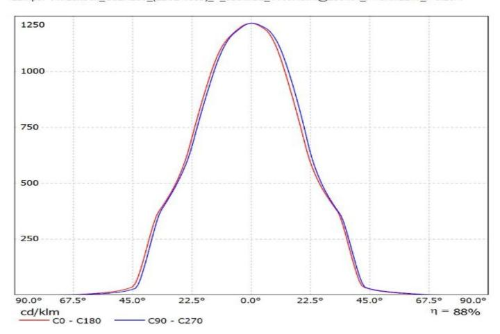
Luminaire: Ledil FN15268\_ANGELETTE-M-RZ\_(CoB1208+TE) Lamps: 1 x Luxeon\_CoB1208\_+\_2213130-2\_+\_2213194-1\_1055.15lm@250mA\_CCT=3000K\_P=8.3007W\_I=0.25A
