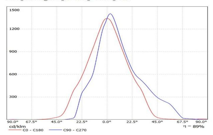
Luminaire: Ledil C14346\_ANGELETTE-WAS\_(CoB1208+TE) Lamps: 1 x Luxeon\_CoB1208\_+\_2213130-2\_+\_2213194-1\_1062.11Im@250mA\_CCT=3000K\_P=8.3007W\_I=0.25A
