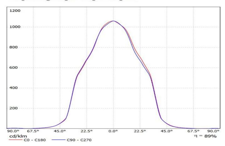
Luminaire: Ledil F14534\_ANGELETTE-WW\_(CoB1208+TE) Lamps: 1 x Luxeon\_CoB1208\_+\_2213130-2\_+\_2213194-1\_1062.11Im@250mA\_CCT=3000K\_P=8.3007W\_I=0.25A
