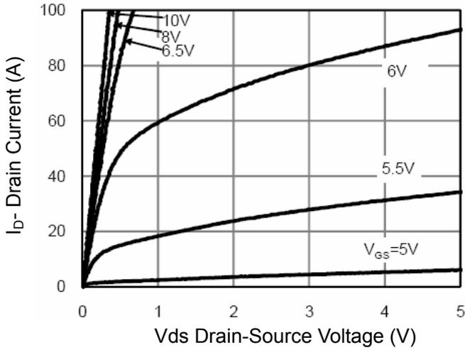
Figure 1 Output Characteristics
