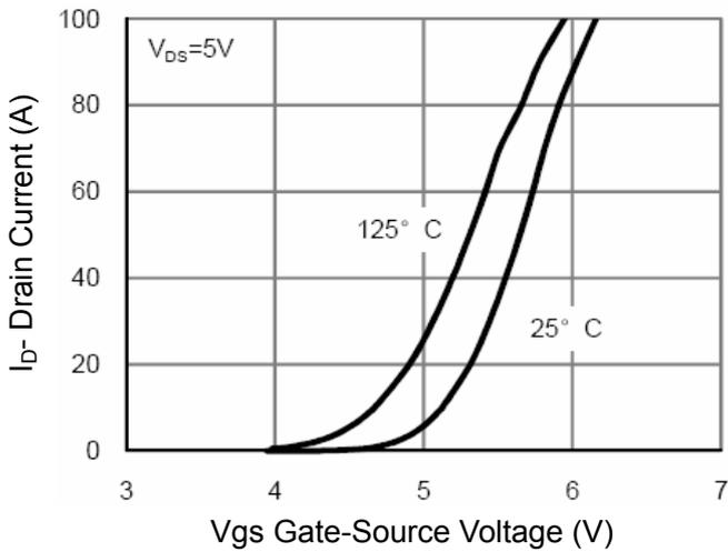
Figure 2 Transfer Characteristics
