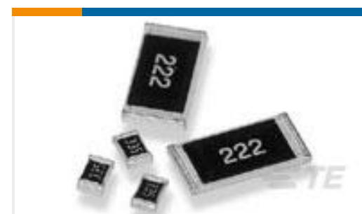
TE Part #1623502-1 CRG1206 1% 3K3
