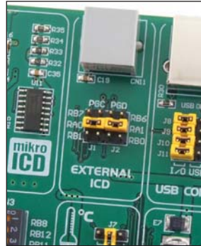
Figure 5-3: Pins RA0 and RA1 are used for programming
