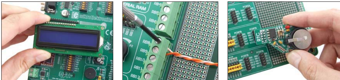
Figure 1-3: Placing additional modules on the board
