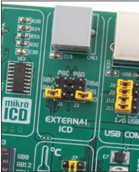
Figure 5-1: ICD connector (default position)
