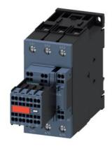
power contactor, AC-3e/AC-3, 65 A, 30 kW / 400 V, 3-pole, 20-33 V AC/DC, 50/60 Hz, with integrated varistor, auxiliary contacts: 2 NO + 2 NC, main circuit: screw terminal, control and auxiliary circuit: spring-loaded terminal, size: S2, captive auxiliary switch
