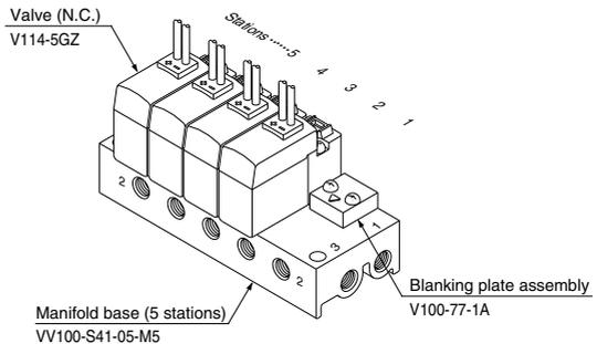
VV100-S41-05-M5 ..... 1 set (Type S41, 5 station manifold base part no.)
