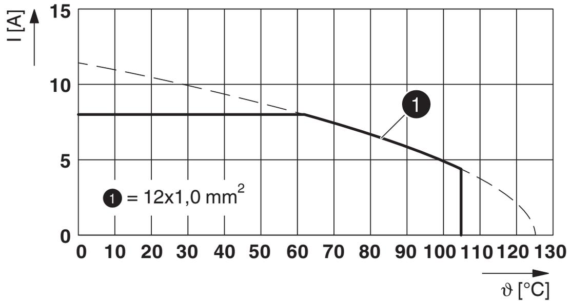
$I$  = current strength,  $\vartheta$  = ambient temperature, 12x 8 A
