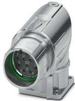
M23, Device connector front mounting, series: M23 PRO, angled rotatable, shielded: yes, for standard and ONECLICK fast locking system, No. of pos.: 12, Direction of rotation: Counter direction, contact connection type: Socket, Crimp connection, flange dimensions: 28 mm x 28 mm, coding: N, Item is lead-free in accordance with RoHS II without Exemption 6c (Pb < 0.1 %)
