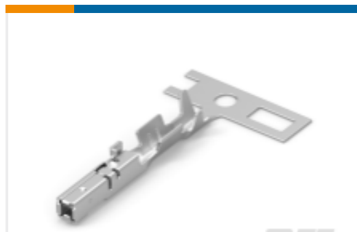
TE Part #1674311-7 0.64 III RCPT 3 Serrations Pre-Tin
