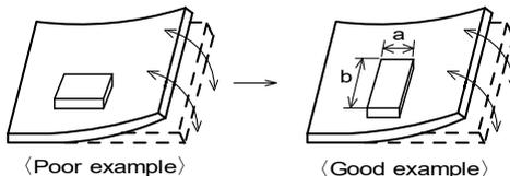
(2) Components location on PCB separation
