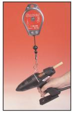
TEC SB/1200 Spring Balancer If the TEC 650 is being used for repetitive work over a work surface, then the TEC SB/1200 Spring Balancer is an economic tool support system with easily adjustable tension control. Capable of supporting tools up to 1.5 kilos in weight, it has a maximum extended cord length of 1.6 metres. Designed to minimise operator fatigue, it also increases productivity and
