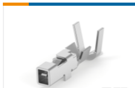
TE Part #1903114-2 Contact: Component To Wire; 3-5A, 30-18 Wire Size
