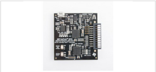
CAPTIVATE-PGMR MSP430 CapTivate MCU Programmer Board Image
