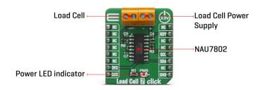
The NAU7802 have many built-in features, which enable high performance applications with very low external parts count. Additionally, both operating current and standby current are very low, and many power management features are included. These enable powering only those elements of the chip that are needed, and also, to operate at greatly reduced power if the full 23-bit ENOB performance is not required.
