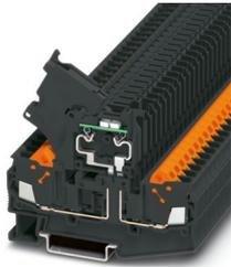
Fuse modular terminal block, fuse type: Glass / ceramics / ..., fuse type: G / 5 x 20, nom. voltage: 500 V, nominal current: 6.3 A, connection method: Quick connection, 1 level, Rated cross section: 1.5 mm<sup>2</sup>, cross section: 0.5 mm<sup>2</sup>- 2.5 mm<sup>2</sup>, mounting type: NS 35/7,5, NS 35/15, color: black
