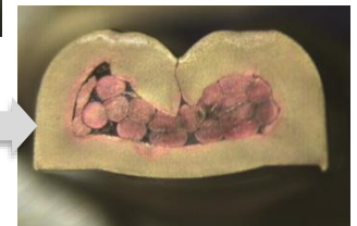
Gross deformation of crimped terminal resulting from material buildup in crimper.
