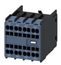
auxiliary switch, on the front, 1 NO + 3 NC, 31/32, 41/42, 51/52, 63/64, current path: 1 NC, 1 NC, 1 NO, spring-loaded terminal, for contactors 3RT2 and contactor relays 3RH2
