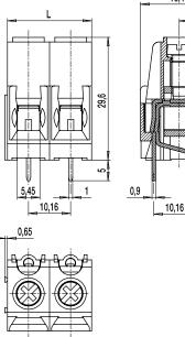
Series 158-A is particularly designed for high voltages and strong currents. A terminal space for solid wires of up to 16 mm<sup>2</sup> or for flexible wires of up to 10 mm<sup>2</sup> is characteristic for this series. Two solder pins per pole ensure safe connection to the PCB.
