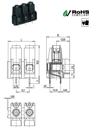
Series 159-A is particularly designed for high voltages and strong currents. A terminal space for solid wires of up to 16 mm<sup>2</sup> or for flexible wires of up to 10 mm<sup>2</sup> is characteristic for this series. Two solder pins per pole ensure safe connection to the PCB.
