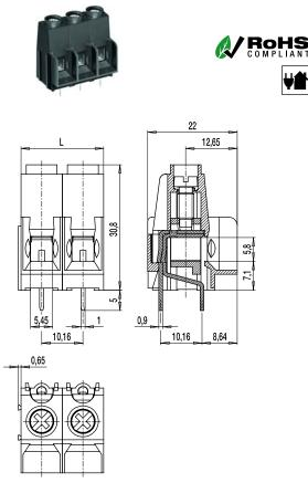
Series 158-A is particularly designed for high voltages and strong currents. A terminal space for solid wires of up to 16 mm<sup>2</sup> or for flexible wires of up to 10 mm<sup>2</sup> is characteristic for this series. Two solder pins per pole ensure safe connection to the PCB.
