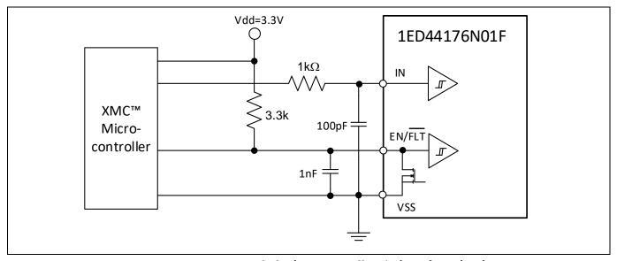
Figure 3 Recommended micro-controller I/O interface circuit
