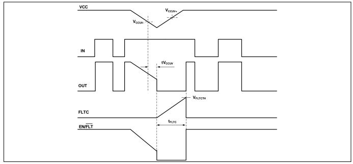
Figure 9 Vcc under voltage protection case one
