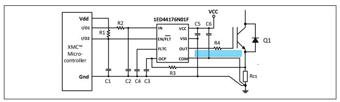
Figure 7 Recommended wiring of bypass capacitors
