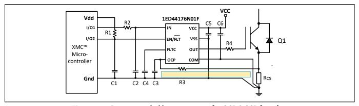
Figure 6 Recommended layout pattern for OCP & SCP function
