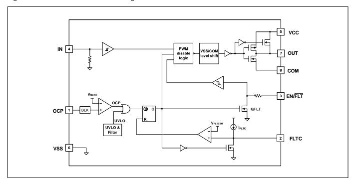
Figure 1 Internal block diagram
