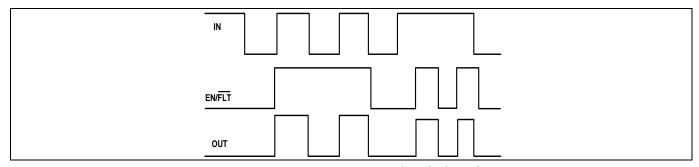
Figure 14 Input/output/enable pins timing diagram
