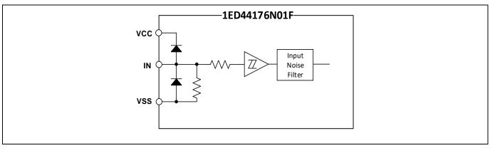
Figure 4 Simplified input structure diagram of 1ED44176N01F
