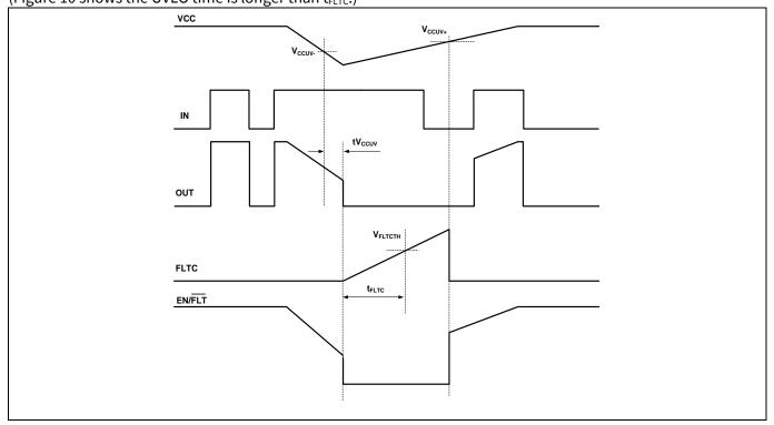
Figure 10 Vcc under voltage protection case two
