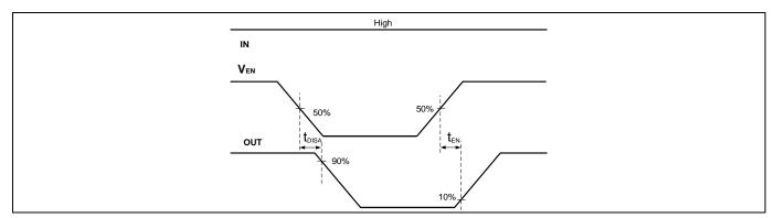
Figure 15 EN pin switching time waveform
