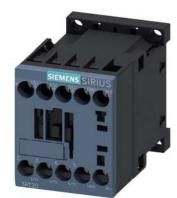
power contactor, AC-3e/AC-3, 12 A, 5.5 kW / 400 V, 3-pole, 24 V DC, 0.7-1.25\* Us, auxiliary contacts: 1 NO, screw terminal, size: S00, suitable for PLC outputs, not expandable with auxiliary switch
