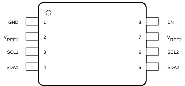
Figure 5-2. DCU Package 8-Pin VSSOP (Top View)
