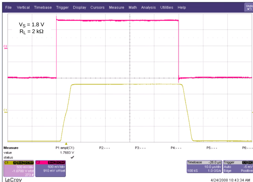
Figure 18. Small Signal Noninverting Response
