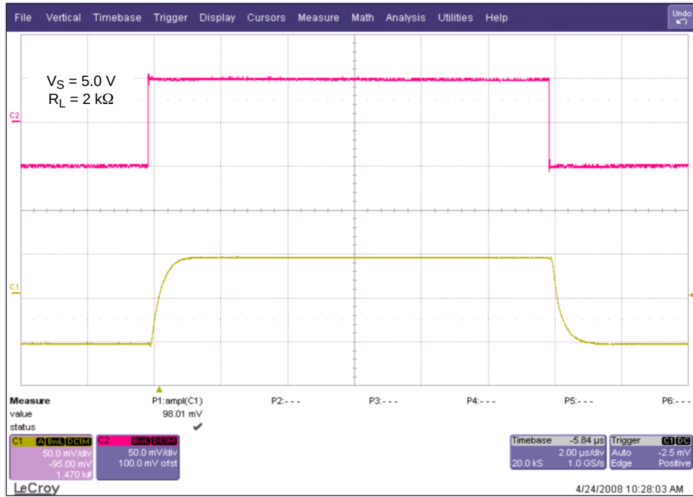
Figure 18. Small Signal Noninverting Response
