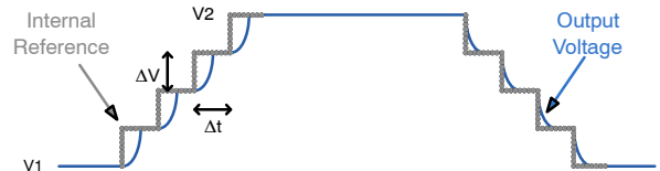
Figure 44. DVS in Forced PPWM Mode Diagram
