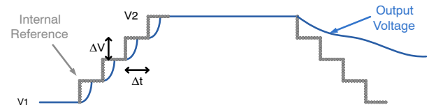
Figure 45. DVS in Auto Mode Diagram
