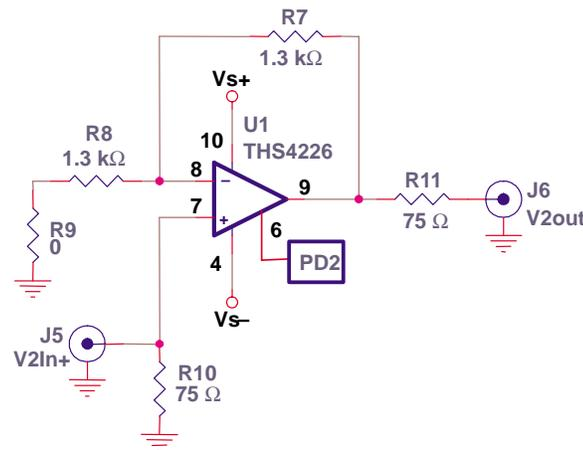
This is a common amplifier configuration used to drive transmission lines. The 75-Ω resistor in series with the output is for connection to a video instrument or circuit.
