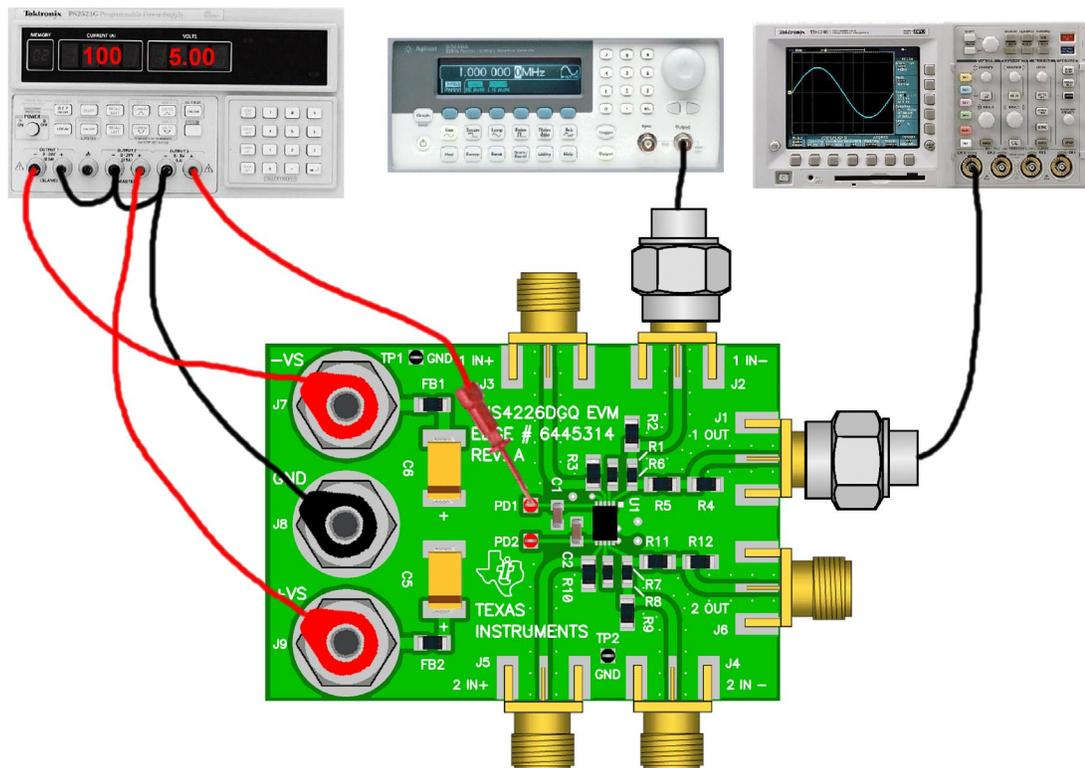
Figure 2-1 shows the connections to measure output 1 while a signal is inserted into the channel 1, noninverting input of the EVM. If the oscilloscope input is connected to J1, and the signal source is connected to J2, EVM channel 2 is also configured for a noninverting signal path.
