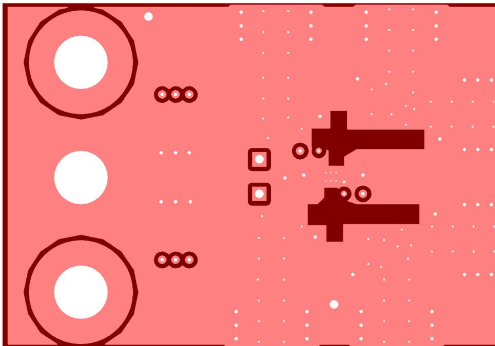
Figure 4-3. Internal Plane (Layer 3) Power Plane7
