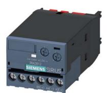
electronic timing relay, off delayed, with control signal and semiconductor output, time range 0.05-100 s, 24-240 V AC/DC, 50/60 Hz, varistor for attenuation of the contactor coils integrated, screw terminal, can be snapped onto the front on contactors 3RT201 / 3RT202 and auxiliary contactors 3RH2
