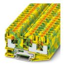
Ground terminal, number of connections: 3, connection method: Push-in connection, Rated cross section: 10 mm², cross section: 0.5 mm² - 16 mm², mounting type: NS 35/7,5, NS 35/15, color: green-yellow
