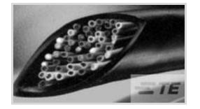
Primary Product Color: Black Wall Type: Single Wall Expanded Inside Diameter (Min): 25.4 mm [1 in] Recovered Inside Diameter (Max): 14.5 mm [.571 in] Shrink Ratio: 1.75:1
