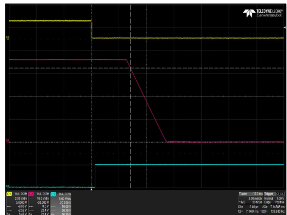
Figure 39: LCM300U Turn Off Characteristic via INH_EN Load: Io = 8.4A (36V), I SB = 2A (5V) Ch 1: INH_EN Ch 2: Vo Ch 3: G_DCOK_C
