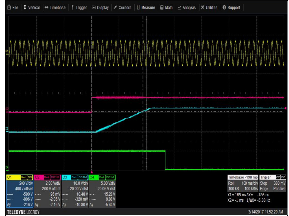
Figure 2: LCM300L Turn-on delay via INH_EN Vin = 90Vac Load: I O = 25A (12V), I SB = 2A (5V) Ch 1: AC Mains Ch 2: INH_EN Ch 3: V O Ch 4: G_DCOK_C
