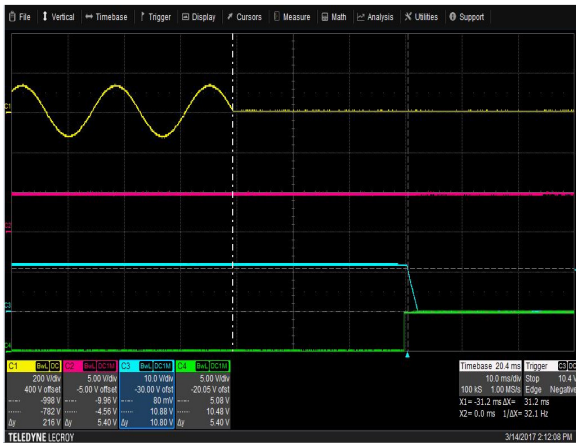
Figure 3: LCM300L Hold-up Time Vin = 90Vac / 47Hz / 0° Load: I O = 25A (12V), I SB = 2A (5V) Ch 1: AC Mains Ch 2: V SB Ch 3: V O Ch 4: G_DCOK_C
